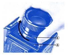
While aligning the two alignment dots (A & 4), insert lens into camera body. Then twist lens clockwise until it clicks and locks into place.
