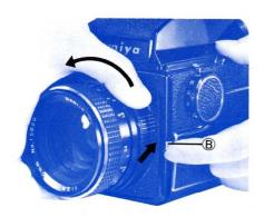
While depressing the lens release button (B), grasp the part of the lens barrel that has the depth-of-field scale and alignment dot (4), and twist the lens counterclockwise until it stops. Then lift out.
